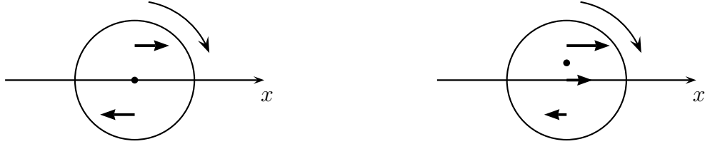
Figure 2: A rotating disk, in its center-of-momentum frame (left), and moving as a whole to the right (right — schematically drawn, no relativistic effects shown). The centroid, in each case, is marked by a dot.
